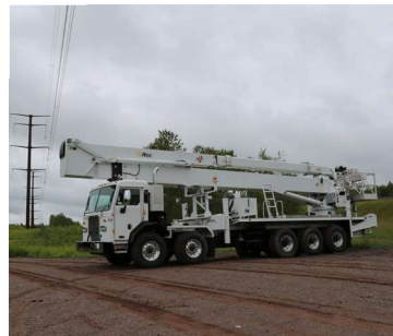
OPTIMIZED BOOM DESIGN COMPLIES WITH FEDERAL BRIDGE FORMULA ON FIVE AXLE CHASSIS
